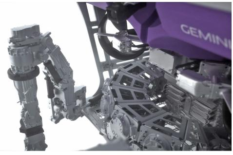
in standard operating conditions. These StationKeep performance enhancements provide an extremely stable platform from which high-precision intervention tasks can be performed by the GEMINI® ROV without the need to anchor and stabilize the ROV by "grabbing on" to the subsea asset. The accuracy of Schilling Robotics' StationKeep mode is unmatched in its ability to maintain vehicle position within a 25- mm watch circle in currents in excess of 2 knots.
