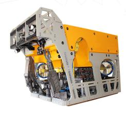
The Heavy Duty (HD) system is an advanced design ROV with class leading performance, reliability, and maintainability. Configured with a Tether Management System (TMS) or in Freefly mode, the HD features innovative frame design and modular sub-systems coupled with a state-of-the-art control system. These attributes make the HD an optimum choice for IMR, drill support, heavy-duty construction operations as well as a vehicle to support ocean research, salvage and military scopes.
