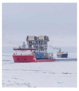
TechnipFMC and its partners confronted the site's freezing and isolated conditions by choosing a modular construction approach, contracting with 10 Asian fabrication yards to build 142 modules and 365 pre-assembled pipe racks weighing more than 480,000 tonnes. Yamal LNG became one of the largest modular construction projects in the world.
