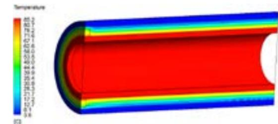
Thermal design - computational fluid dynamics (CFD)
