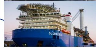
G1200 S-Lay vessel to install rigid pipelines
