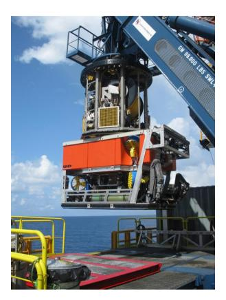
It delivers the performance and efficient hydraulic power required in an ultra-heavy, work-class ROV. The rugged and powerful system is de signed to accommodate the growing market for ultra-heavy tasks, such as suction pile installation, flying lead installation, and other applications that benefit from re-directing power to tooling operations.
