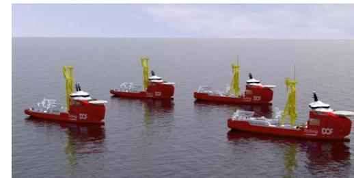
Four Flexible Pipe Lay Vessels
