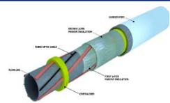
**Electrically Trace Heated Pipe-in-pipe**
