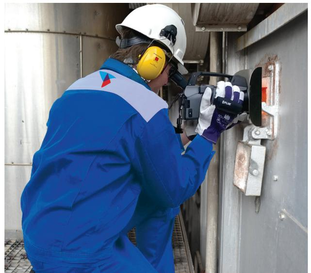
The quick assessment is done with data provided by an infrared camera.
